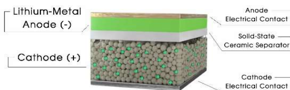
Figure 3. Solid-State Lithium-Metal Battery Structure [11]
