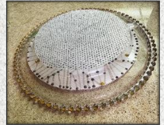
Final layer with hybrid 3D-printed adhesive micropattern suction cups,
