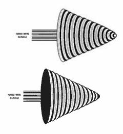
The next two implant concepts use processes similar to those in the manufacture of integrated circuits. The third implant design built upon the previous conical concept but used concentric rings of graphene in place of the wrapped nanowires. This is the implant that we proceeded with, and is described in the Future Technology section.
